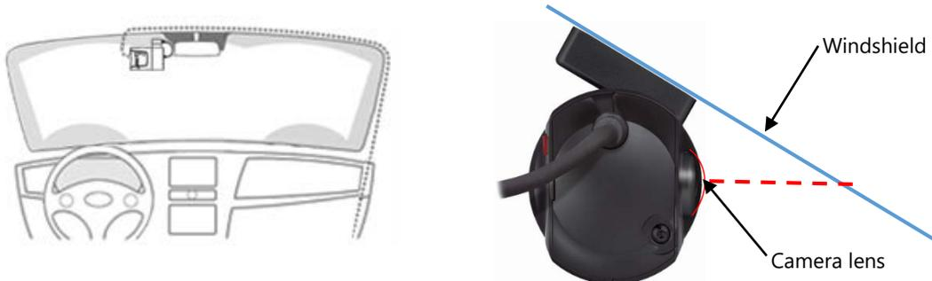
**IMPORTANT:** Make sure that the glass is clean and dry before attaching. Hold the camera in position with firm pressure for 30 seconds. The glass temperature should not be too hot or cold. Please install in moderate temperature (recommended between 50°F ~ 80°F)
