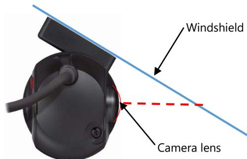
**IMPORTANT:** Make sure that the glass is clean and dry before attaching. Hold the camera in position with firm pressure for 30 seconds. The glass temperature should not be too hot or cold. Please install in moderate temperature (recommended between 50°F ~ 80°F)
