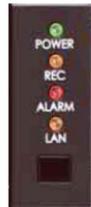
At power up, the **POWER** LED will illuminate immediately and the CRX will go into system check. Once device is operational, the **REC** LED will also illuminate. This usually takes about a minute but in some cases, the device may need to reboot in which case it will take about 5 minutes.
