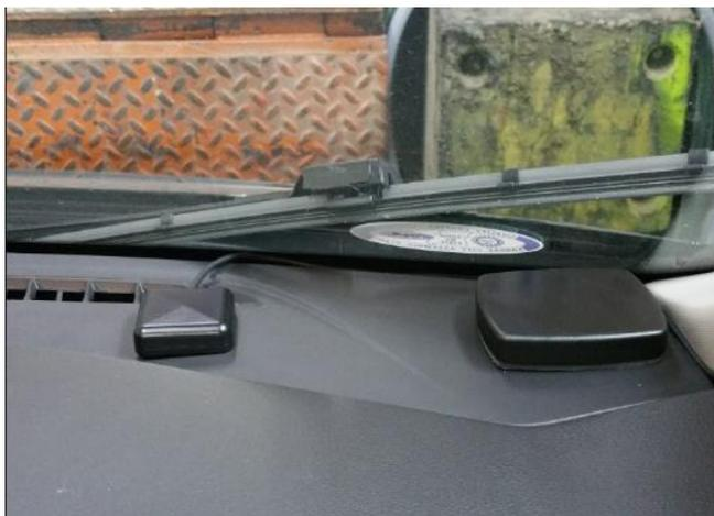
**CRX GPS and LTE antenna properly installed on the Vehicle Dash**
