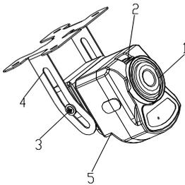
1. Attach the mounting bracket (4) to wall or ceiling, as required. Use the supplied screws to fix camera (5) in position ~ a firm mounting surface is essential for a stable installation.
