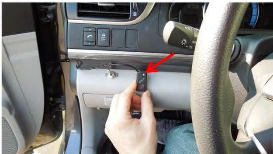
5) Run remote & camera cable(s) and secure in headliner or other area so no cables are exposed. Use provided wire clips if necessary. Cables should enter through rear of the locking case.
