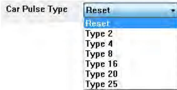
Before using “Car Pulse Type”, connect the White (Speed pulse) cable to the speed pulse line on your car. Please consult your car manufacturer or a car repair shop regarding this connection.
