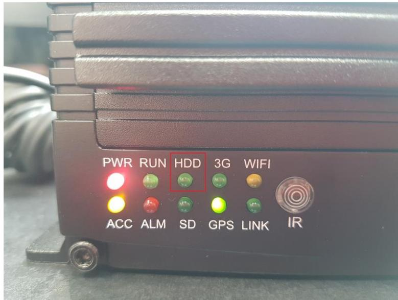
If the LED is not flashing, it will be best to check the Hard Drive Status in the settings on the DVR. Using the DVR remote control, press the "**Menu**" button to enter the main menu. You will now need to enter your admin password. By default this is "**6666**".
