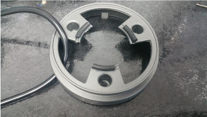
After drilling, feed through the camera wires into the base, as shown above. Then screw back the remaining screws.
