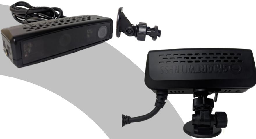
The **SmartWitness DDC-200** is the world's most advanced fatigue detection and driver distraction alert camera. The detection is focused on a driver's physical indicators, such as gaze direction, facial features, etc. that reflect a driver's overall alertness, and produces a sound alerting system in case a driver gets distracted or is falling asleep. The **DDC-200** allows for day and night detection with the use of infrared light even through dark eyewear.
