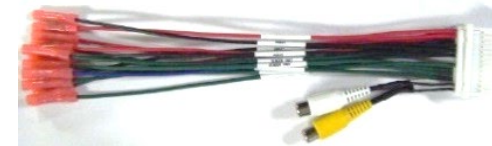
Alarm I/O Trigger Harness and A/V Output for connecting an LCD monitor
